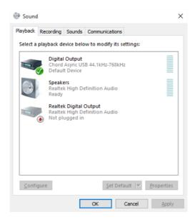
Here you have a list of the connected audio devices. Dave is identified as a digital output device with the 'Chord Async USB 44.1kHz - 768kHz' driver installed - shown at the top of the list here. Highlight the digital output and then click set default at the bottom of the screen. Then click ok to close the window.
