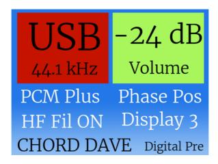
Display mode 4 is largely similar to display mode 1. However, after 30 seconds, the screen will enter 'screensaver mode' and will shut off until a function button is pressed.
